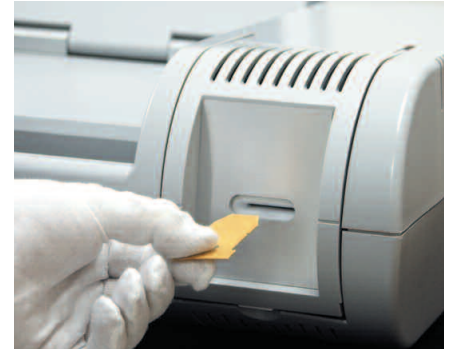
Inserting a sample trap initiates detection.
