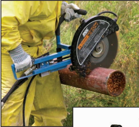
S16 Cutting Steel Pipe w/ Abrasive Blade
